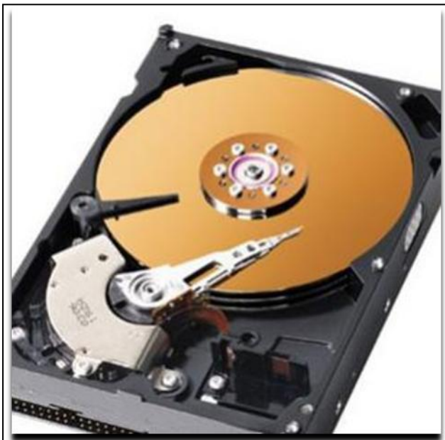
Hard disks store digital information in a relatively permanent form. Figure (C.1).
